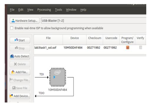
Note that the device indicated here is the one on the DE10 board: 10M50DAF484. Click the **Start** button.
